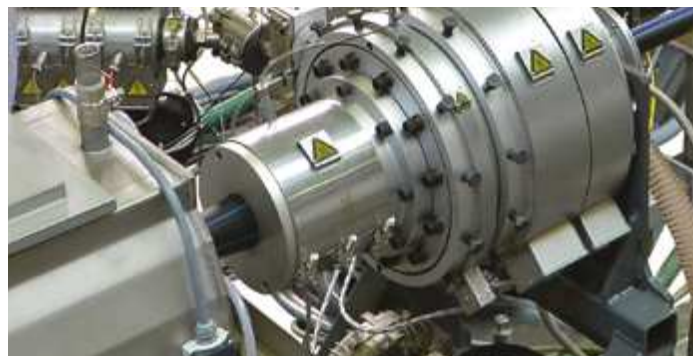
Pipe head for pipe-in-pipe extrusion
