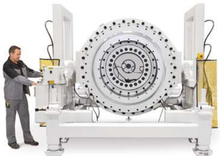
Spider double pipe head for 1,200 mm PVC pipe
