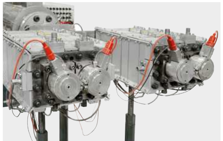
Spider 50-4 pipe die for quadruple strand extrusion of U-PVC pipes
