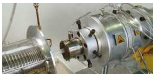
Pipe head for aluminium pipe extrusion
